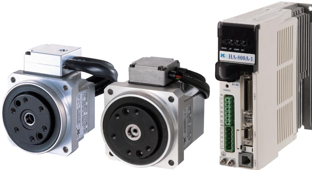
This is the AC servo actuator consisting of HarmonicDrive® integrated with a compact/flat AC servo actuator. This actuator has a uniquely compact shape and a hollow structure that penetrates through the actuator located at the center. By passing the wire, pipe, laser light, and others through the actuator, machines and devices can be simplified. You can select the built-in encoder from the incremental and absolute types. Combination with the dedicated driver achieves even more accurate control.
